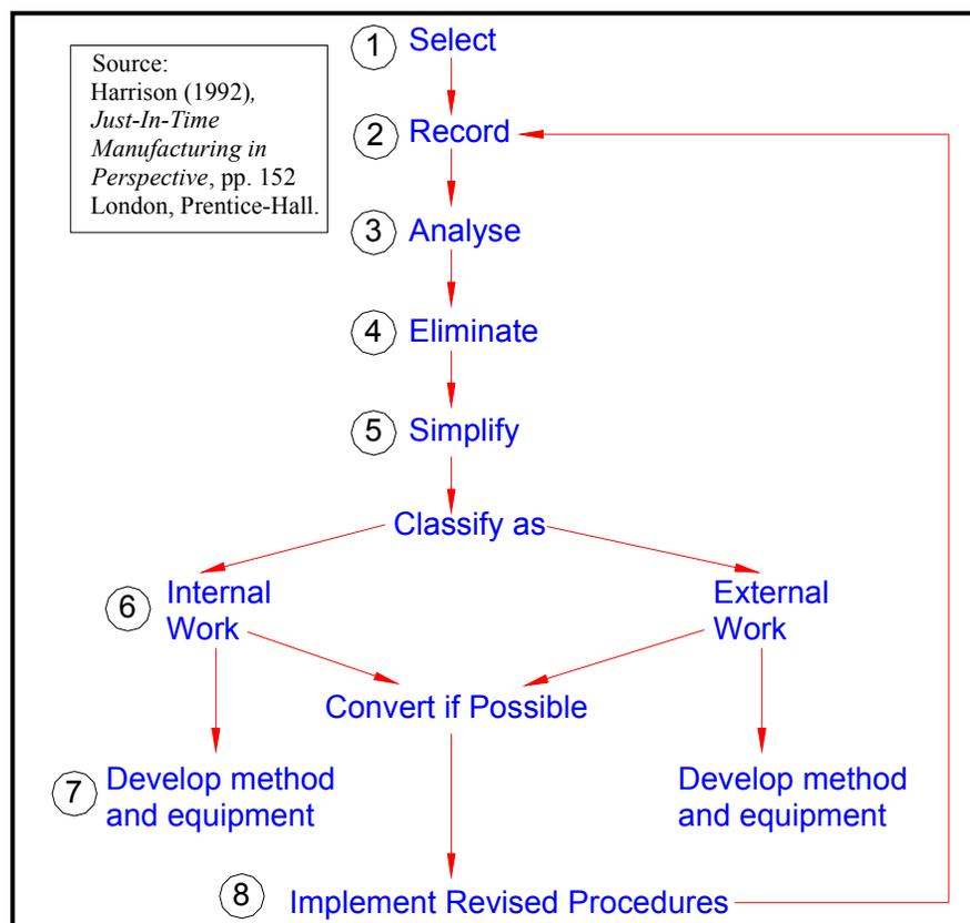
**Figure: Eight Steps to Setup Reduction (Harrison, 1992)**
